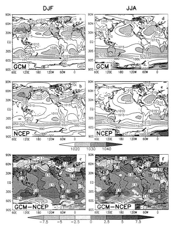
Fig. 5. Climatological sea surface pressure (hPa): DJF (a) CPTEC-COLA AGCM and (b) NCEP-NCAR reanalysis, and JJA (d) CPTEC-COLA AGCM and (e) NCEP-NCAR reanalysis. (c), (f) The differences between the model and observations.
