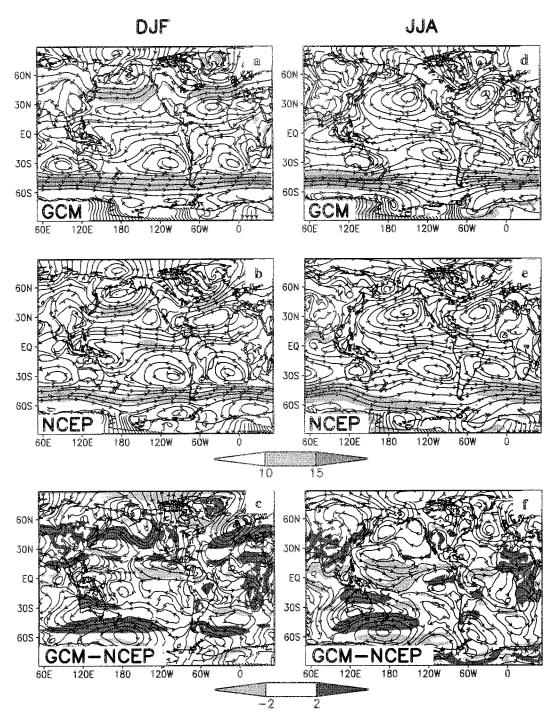
Fig. 6. Isolines and magnitude of climatological wind field at 850 hPa (m s $^{-1}$ ): DJF (a) CPTEC–COLA AGCM and (b) NCEP–NCAR reanalysis, and JJA (d) CPTEC–COLA AGCM, and (e) NCEP–NCAR reanalysis. (c), (f) The differences between the model and observations. The magnitudes are shaded.
