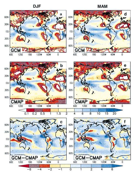
FIG. 4. Climatological precipitation (mm day<sup>-1</sup>): (a) DJF CPTEC–COLA AGCM, (b) DJF CMAP, (d) MAM CPTEC–COLA AGCM, (e) MAM CMAP, (g) JJA CPTEC–COLA AGCM, (h) JJA CMAP, (j) SON CPTEC–COLA AGCM, and (k) SON CMAP. (c), (f), (i), (l) The differences between model and observations.
